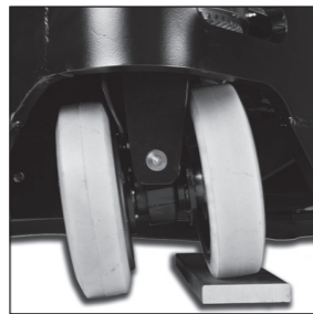
Independent steering motors and braking systems for support wheels
